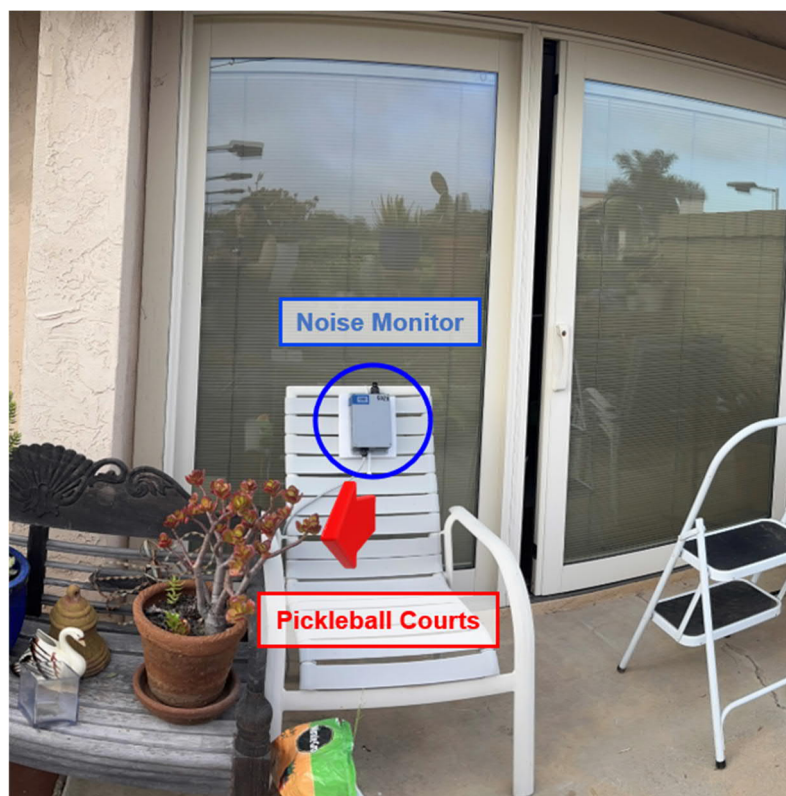
Figure 2 - Noise monitor location, in situ
